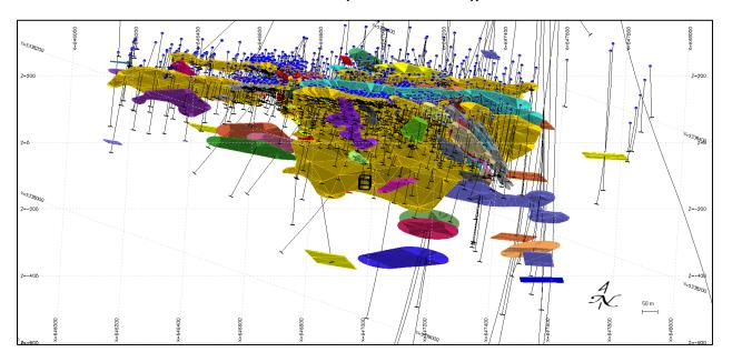
Figure 14-5 Isometric View Looking NNW Showing the Drill Holes, and the Thin, Rich **Veins Model**
