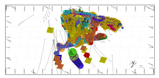
Isometric View Looking SSE Showing the Drill Holes, and the Thin, Rich Figure 14-4 **Veins Model (107 Wireframes))**
