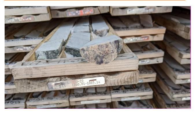
Figure 12-10 GR-20-22 from 1060 to 1065 m with Purple Mineral as Fracture Filling
