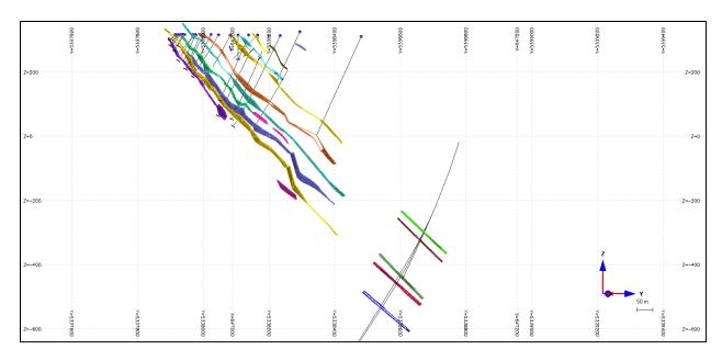
Figure 14-6 Section 34.5 Looking West Showing the Drill Holes, and the Thin, Rich Veins Model
