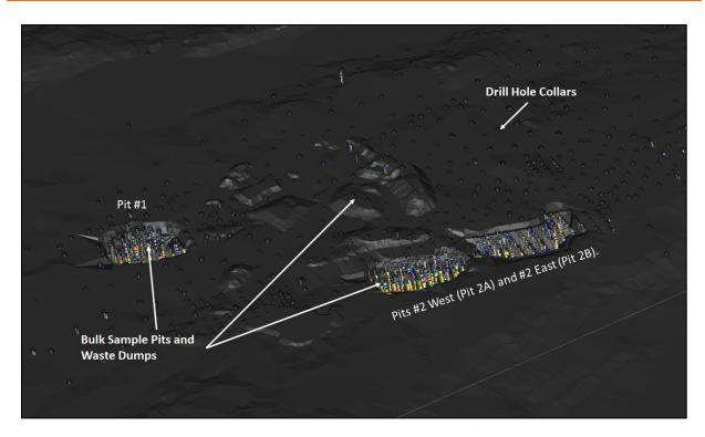
Isometric View Looking Northeast of the Granada Deposit Area Showing Figure 14-2 the Topographic Surface Including Areas of Bulk Sampling
