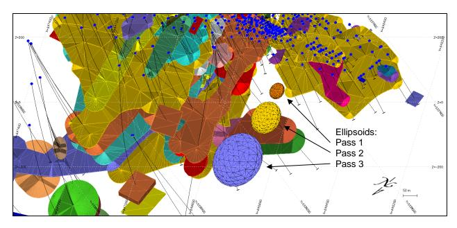
Figure 14-7 Isometric View Looking South-southeast with the Thin, Rich Veins Model and the Pass 1, 2 and 3 Search Ellipsoids
