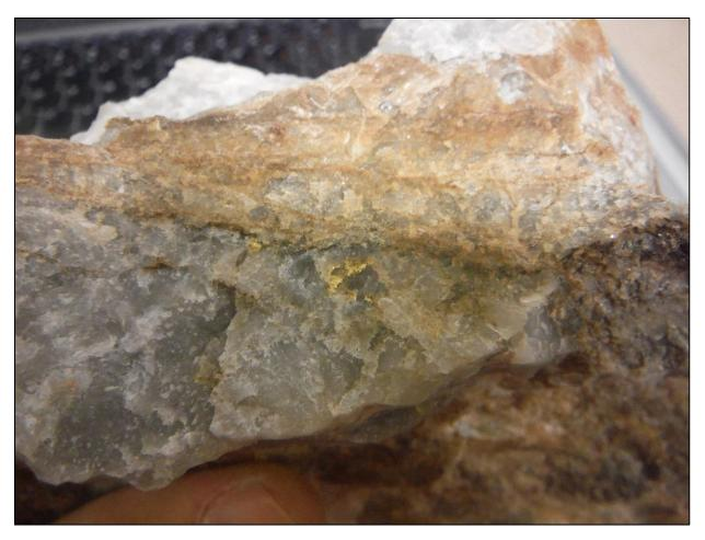
Figure 7-6 Visible Gold Within Smoky Quartz Vein in a Surface Sample
