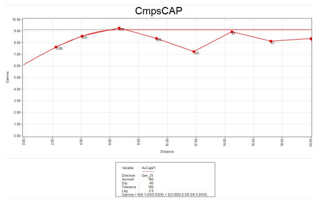
Figure 14-8 Along-the-holes Experimental Variogram and Model
