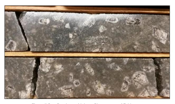
Figure 7-5 Porphyry with large Phenocrysts of Feldspars
