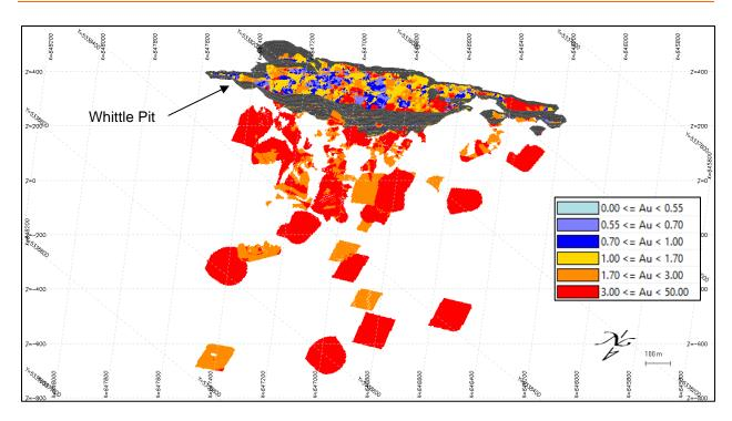
Figure 14-9 Isometric View Looking South-southeast with Block Model. 0,55 g/t Au COG Inside the pit and 2.5 g/t Au COG Under the Pit
