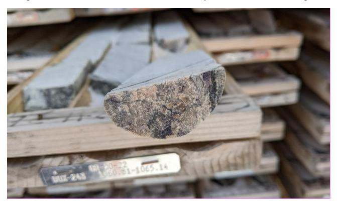
Figure 12-11 GR-20-22 from 1060 to 1065 m with Purple Mineral as Fracture Filling
