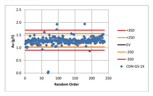
Figure 11-19 Distribution of Standards CDN-GS-1X (Au g/t) used in the 2021 Drilling Campaign
