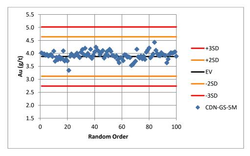
Figure 11-13 Distribution of Standards CDN-GS-5M (Au g/t) (2020 Drilling Campaign)
