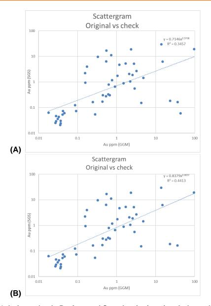
Figure 12-14 Independently Re-Assayed Samples Au (ppm) vs Independent SGS Au (ppm) (A) with and (B) without Sample 7583/61997
