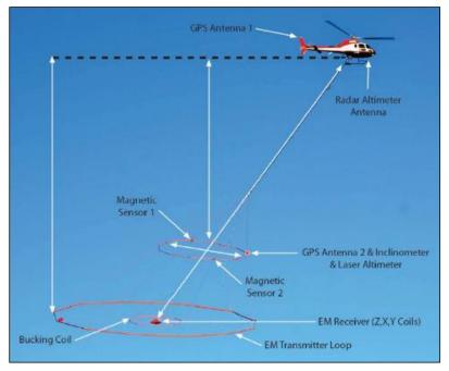
Figure 9.1: Heliborne magnetic and VTEM survey setup layout
