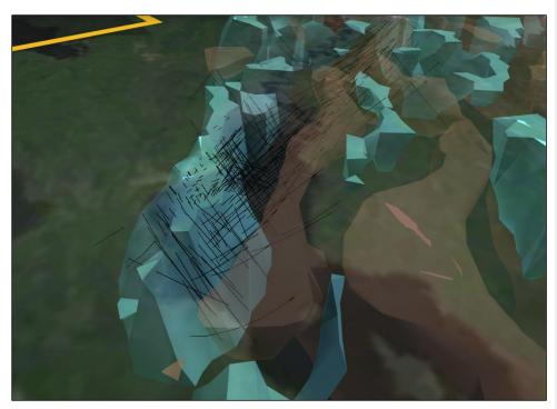
Figure 9.5: 3D view of the Technolmaging inverted magnetic data, looking along the main Moss Gold Deposit towards the northeast (blue and red volumes are picked magnetic low and high anomalies, respectively)
