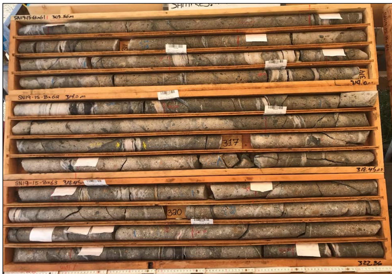
FIGURE 7.14 VEINLET DOMAIN IN DRILL HOLE SN19-15 (309.50 M TO 322.86 M)
