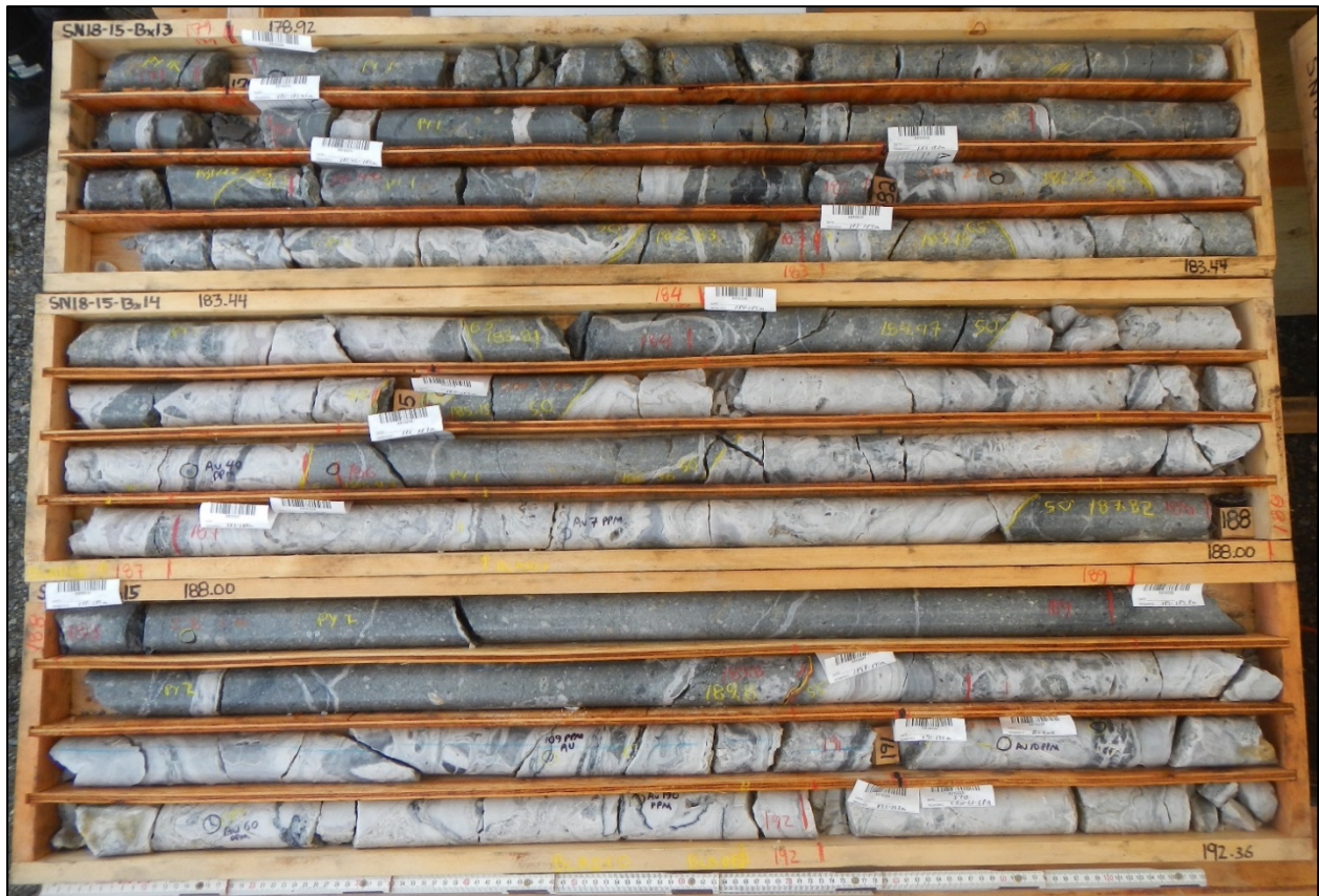
FIGURE 7.8 VEIN ZONE 1A IN DRILL HOLE SN18-15 (178.92 M TO 192.36 M)
