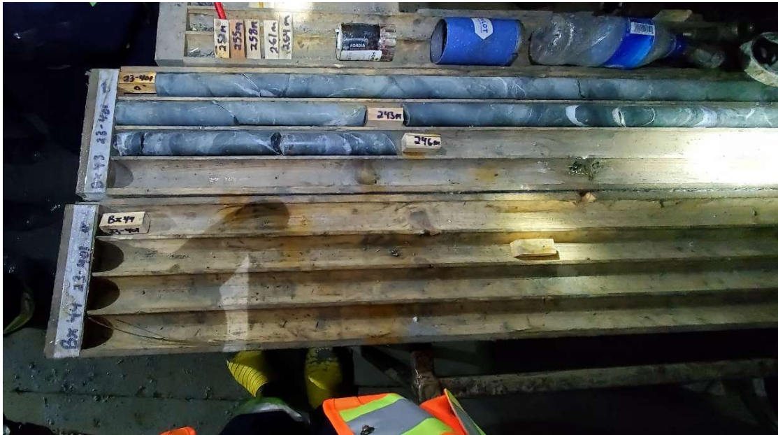
Figure 10.4 – Wooden blocks placed every 3 metres by drill helper
